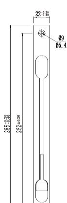
**Flush Bolt** • Manufactured from satin-statinless steel
