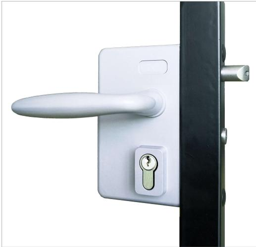
○ This industrial lock is made with an aluminum housing and stainless steel mechanism. We believe this lock should be a standard for all your industrial gates. The 20mm continuous adjustability of the bolts allows a perfect alignment of your locking mechanism. A solid stainless steel deadbolt with a 22mm throw guarantees a secure locking. Standard supplied with aluminum handles and key barrel.
